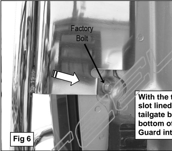
With the top mounting slot lined up under the tailgate bolt, move the bottom of the Taillight Guard into position
