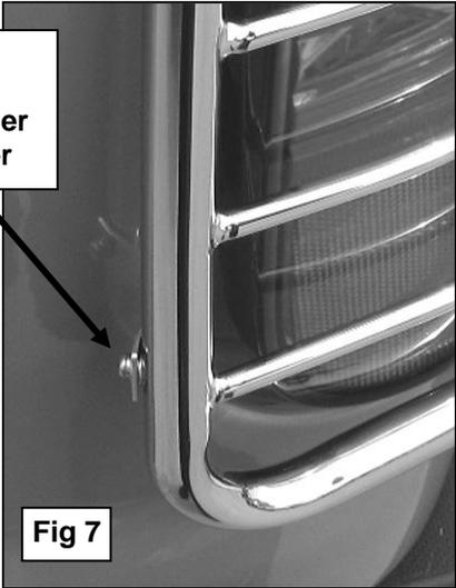
If necessary, gently and evenly bend the mounting bracket into the proper position
