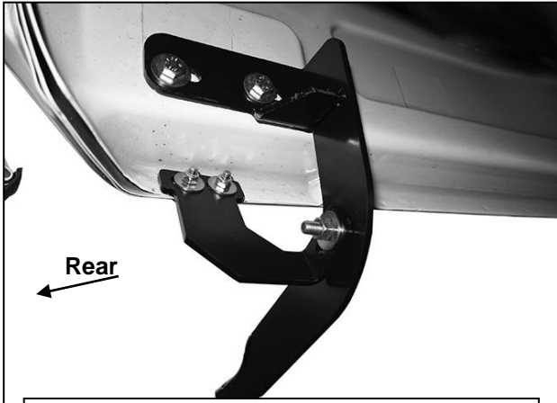
(Fig 16) Driver/Left rear Brackets installed
