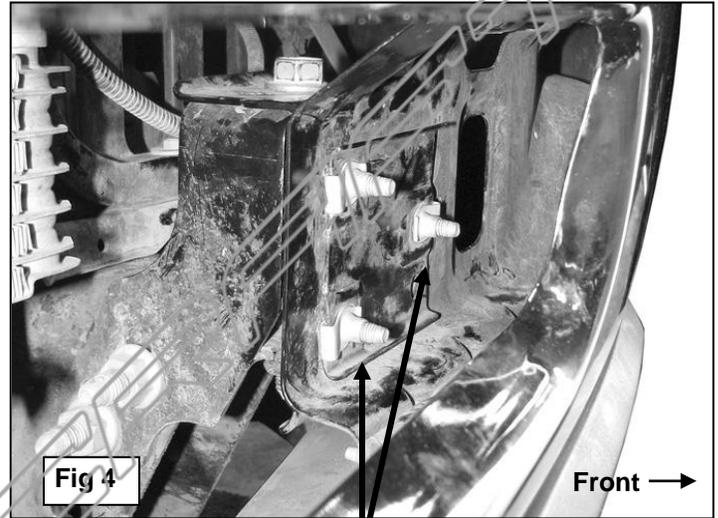
Remove (3) factory hex bolts and cover plate w/clips
