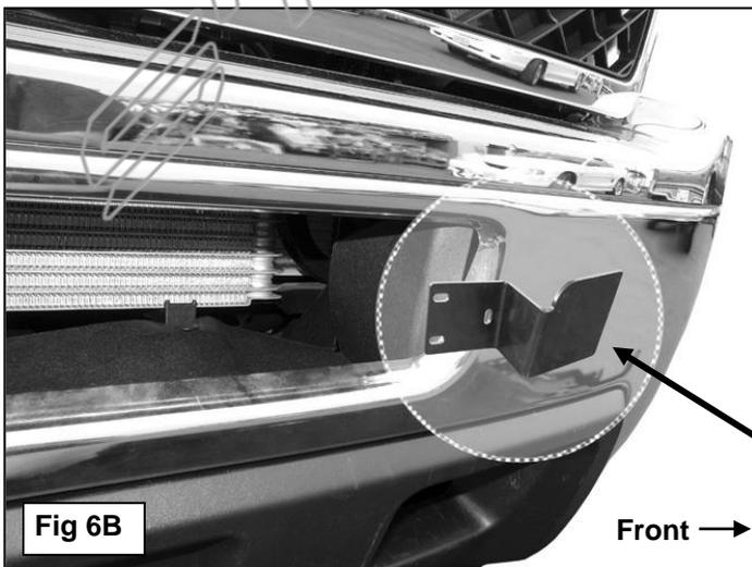
Driver side Support Bracket illustrated to show Bracket position inside against the back of the front bumper
