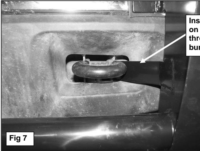
Insert mounting tab on Grille Guard through opening in bumper cover.
