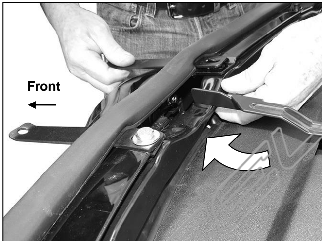
(Fig 9) Hold 8mm Nut Plate up to underside of metal cross member. Attach Top Bracket to Nut Plate, (passenger/right pictured during installation)
