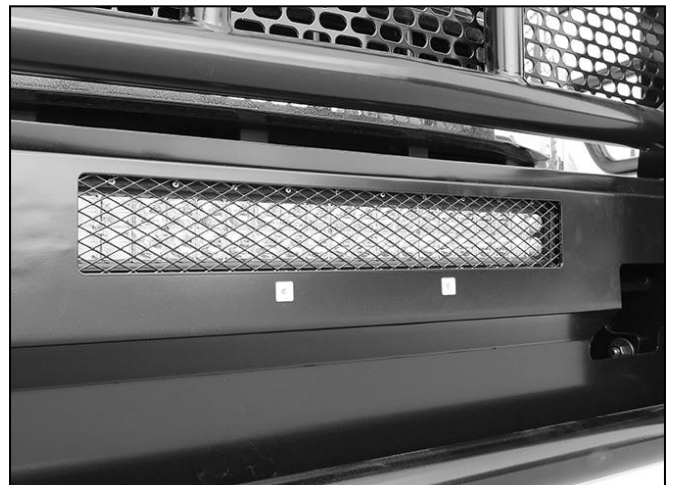
(Fig 14) Push plastic plugs into holes in Bumper for license plate if required. LED bar light pictured installed behind Bumper on non-ecoboost model. LED light installation not recommended on ecoboost models
