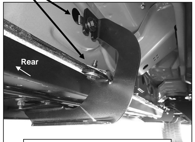
(Fig 10) Driver/left brackets installed
