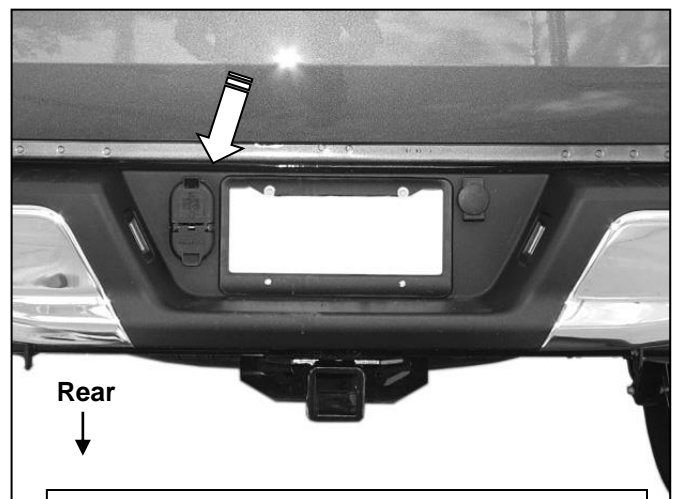
(Fig 2) Unplug and remove 7-wire trailer plug
