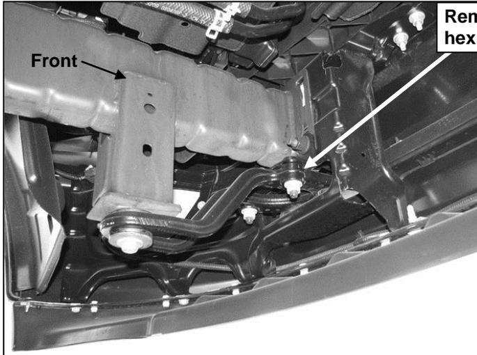
Remove the (2) factory hex nuts from tow hook
