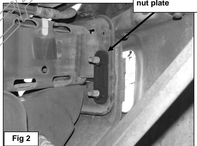
**WARNING!** Do not loosen or remove passenger and driver side bumper mounting bolts at the same time or bumper may move out of alignment or fall off of the vehicle. Only remove the bumper bolts from one side and install one Mounting Bracket at a time.
