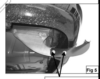
12-1.75mm x 30mm Hex Bolts 12mm Nylock Nuts 12mm Flat Washers
