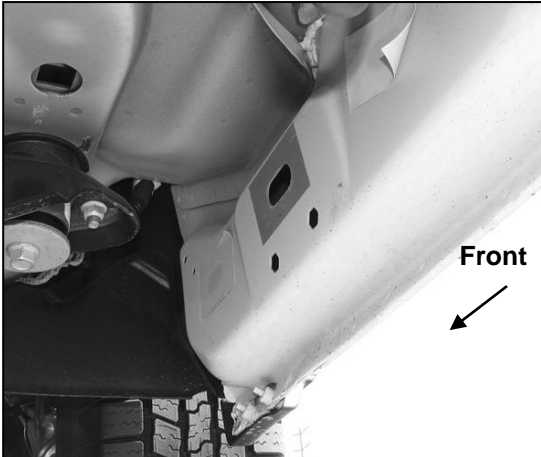
(Fig 1) Passenger/right front mounting location (model without threaded inserts)
