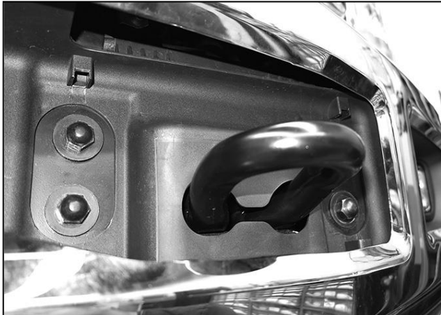
(Fig 6) Remove bumper bolts (driver side pictured)
