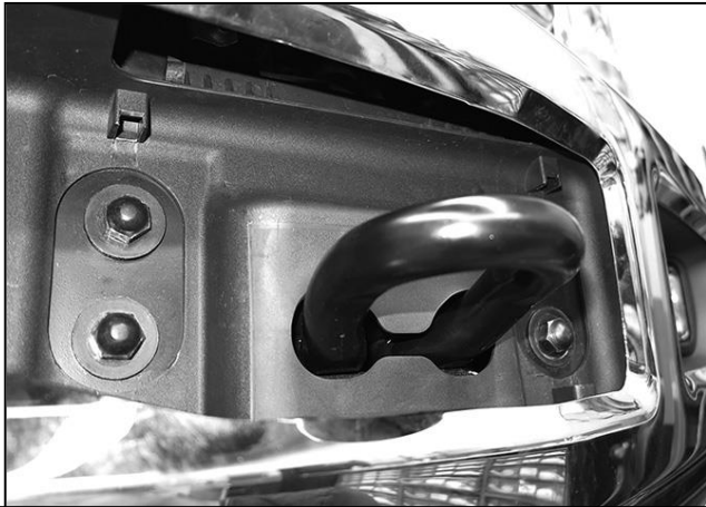
(Fig 6) Remove bumper bolts (driver side pictured)
