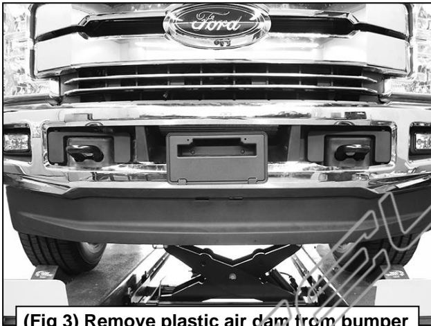
(Fig 3) Remove plastic air dam from bumper
