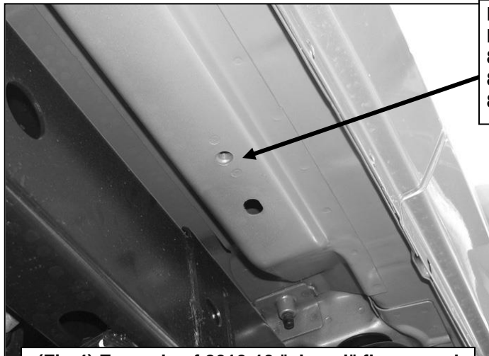
(Fig 4) Example of 2010-13 "closed" floor panel with threaded hole-10mm Nut Plate not required
