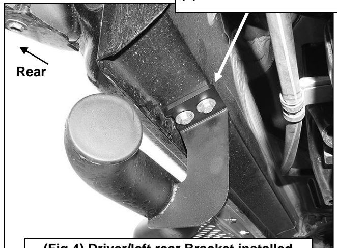
(Fig 4) Driver/left rear Bracket installed
