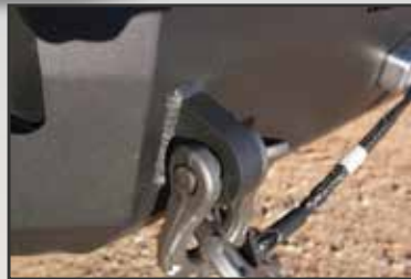
Welded eyelets for shackles
