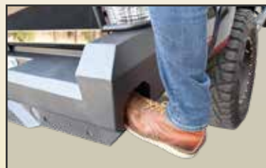
Convenient step for easy bed access built in
