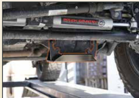
Differential protection with drain plug cutout
