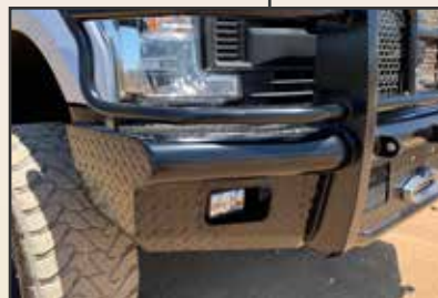
Welded eyelets for shackles. Plus retain your factory fog lights
