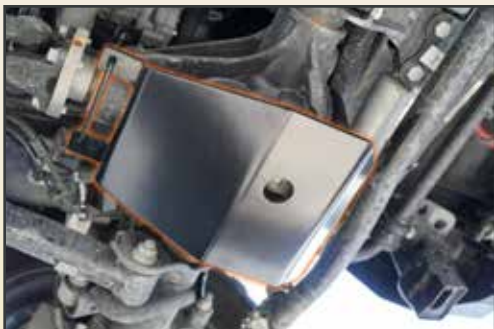
Differential protection with drain plug cutout
