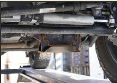
Differential protection with drain plug cutout
