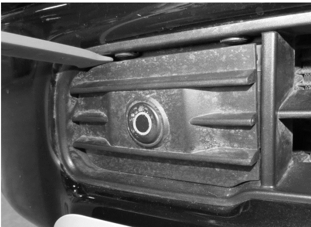
(Fig 4B) Titan XD Only- Use pry tool to remove plastic panel for access to parking sensor
