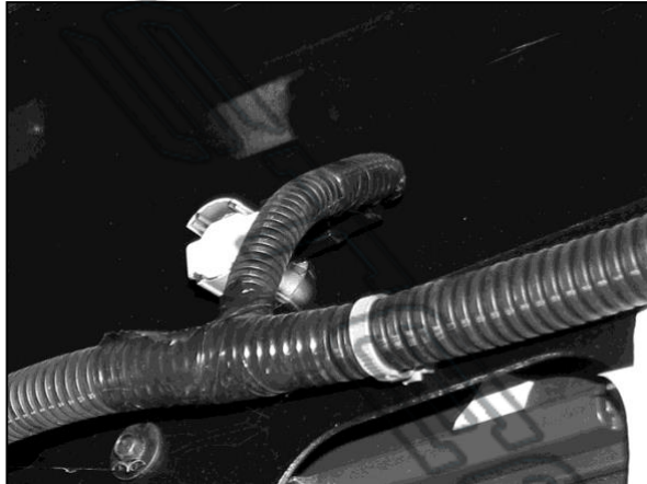
(Fig 3) Unplug and remove OE center sensors from the back of the bumper (example only)
