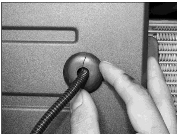
(Fig 12) Push Rubber Grommet on Harness into sensor hole (Bumper used for Example)
