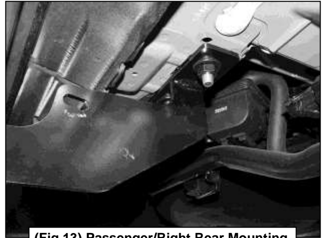
(Fig 13) Passenger/Right Rear Mounting Bracket attached to the (2) Bolt Plates
