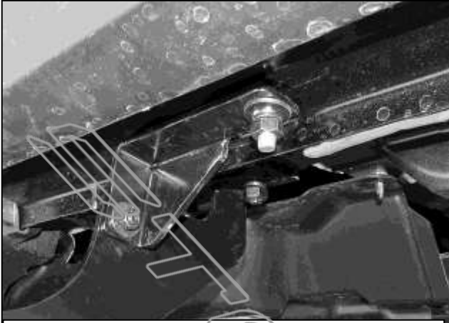
(Fig 16) Passenger/Right Rear Support Bracket attached to the Mounting Bracket and vehicle
