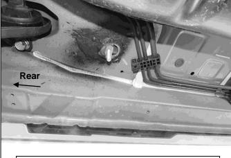
(Fig 10) Insert (1) 10mm Bolt Plate into the rear hole. Thread (1) 10mm Plastic Retainer onto the Bolt Plate to hold it in place
