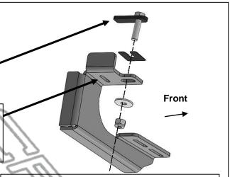
(Fig 9) Attach the Driver/Left Center Mounting Bracket to the center mounting location
