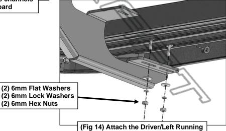
(Fig 14) Attach the Driver/Left Running Board to the Mounting Brackets
