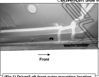
(Fig 1) Driver/Left front outer mounting location
