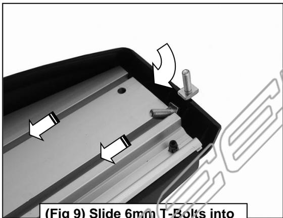
(Fig 9) Slide 6mm T-Bolts into slots at end of Running Board
