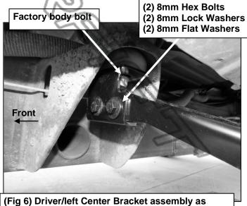
(Fig 6) Driver/left Center Bracket assembly as installed on all model years (except 2014-on 1500)
