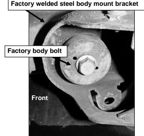
(Fig 1) Driver/left Front Mounting Location
