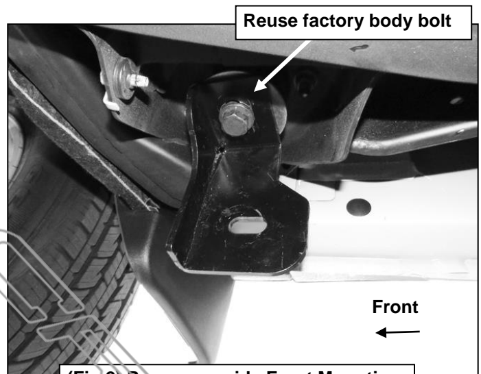
(Fig 2) Passenger side Front Mounting Bracket attached to front body mount
