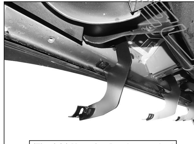
(Fig 3) (1) Mounting Bracket attached to the front mounting location
