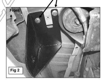
10mm x 30mm Hex Bolt 10mm Lock Washer (2) 10mm Flat Washers 10mm Hex Nut
