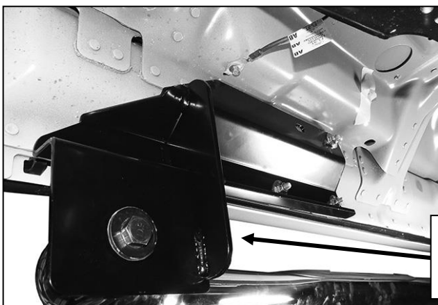
(Fig 5) Passenger side front Bracket installation
