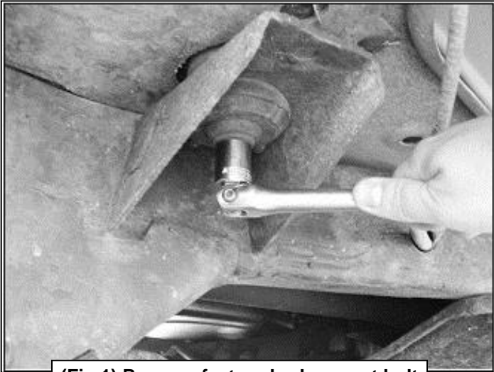
(Fig 1) Remove factory body mount bolt
