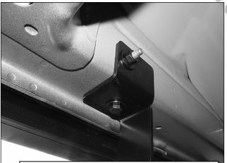
(Fig 6) Driver/Left center Mounting Bracket attached to the center mounting location
