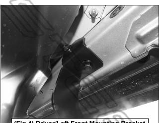
(Fig 4) Driver/Left Front Mounting Bracket attached to the front mounting location
