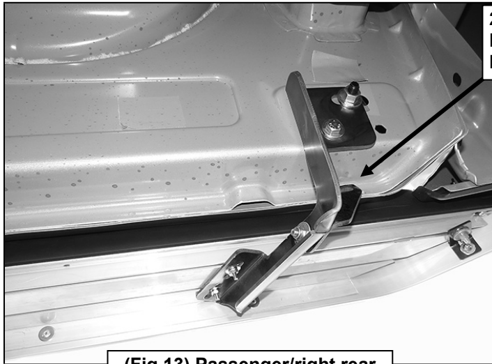
(Fig 13) Passenger/right rear Support Bracket (long)
