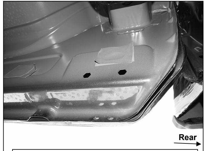
(Fig 7) Passenger/right rear mounting location
