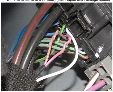
The kit comes supplied with wire taps called "shark taps". Follow the guide below to tap the wire using the "shark tap":
