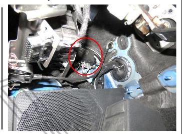
On the black plug of the BCM, identify the Grey/Orange wire and Purple/Orange wire. Connect the Yellow and White signal wires from the Power Step Main Harness (J) using the supplied wire taps (L). (See next page for details)
