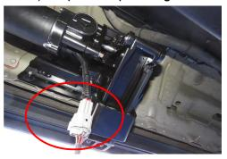
Locate the black BCM (body control module) under the steering wheel, behind the OBD-II Port and to the left side behind the kick panel. BCM module may be detachable.
