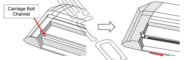
Use the notch in the board's end caps to feed the bolts into the channel.
