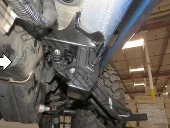
Then fasten the Bolts (J & K), Nylon Lock Nuts (I) and Washers (H). Do not tighten all the way yet. For some vehicles it may be necessary to push or unhook the OE wiring harnesses and re-tie them out of the way using zip ties.
