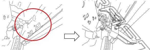
Then fasten Nylon Lock Nuts (I) and washers (H). Do not tighten all the way yet. For vehicles with e-brake cables on the Driver Side, take the rubber sleeve in the kit and slide over the brake line, just behind the bracket assembly, to protect the line from wear. Attach sleeve to line using RTV silicone sealant.
