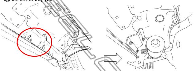
Locate rear mounting points. Apply a plastic insulator (F) to each stud before mounting the Driver Side Rear Bracket Assembly (B). Next, line up rear mounting bracket slots to the studs and place Driver Side/Left Rear Bracket Assembly (B) onto rocker panel.
