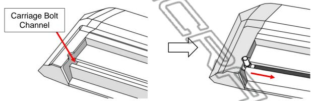
Use the notch in the board's end caps to feed the bolts into the channel.
