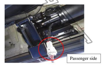
Seal the grommet with RTV Silicone Sealant.
