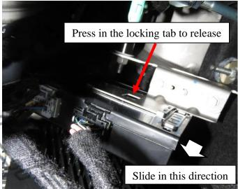
On the black plug of the BCM, identify the blue/green stripe and white/green stripe wires. Connect the High and Low wires from the main harness (J) using the supplied wire taps (L). After successfully connecting the wires, return the BCM back into its place and check that it is secure.
