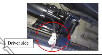
Locate the black BCM (body control module) under the steering wheel, behind the OBD-II Port. Slide the BCM out of the holding bracket by pushing the locking tab in the center and pulling outwards in the direction of the rail for easier access to wires.
