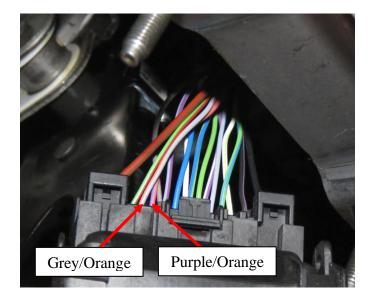
\*NOTE: If board does not move during troubleshooting, flip the CAN Signal High and Low wires.
