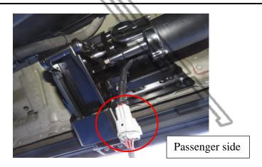
Hide wires and reattach the kick panel with the carpet fully unfurled in its original position. Reattach the door sill panel and check to make sure there are no obstructions or potential snag points around the brake pedal area.
