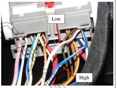
Confirm that the truck is powered off. Connect the High and Low wires from the main harness (J) using the supplied wire taps (L). After successfully connecting the wires, secure the wires so that they do not interfere with the brake pedal. Proceed to step 10.
