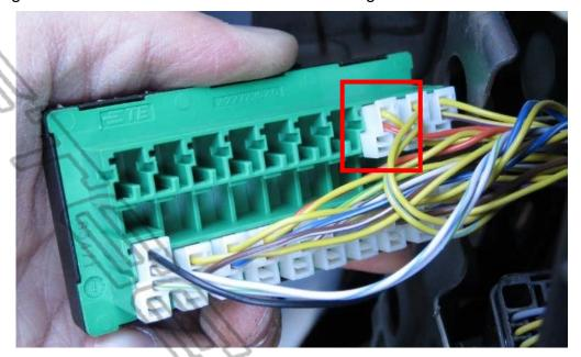
Confirm that the truck is powered off. Connect the High and Low wires from the main harness (J) using the supplied wire taps (L). After successfully connecting the wires, return the module back into its place and check that it is secure on the bracket. Proceed to step 10.
