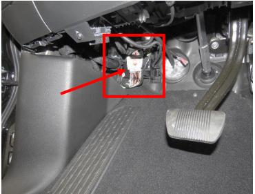
Identify the configuration of the wires on the bottom side of the CAN Bus plug. On the right side, select the twisted pair of wires colored **White** and **Blue with White stripe**.
