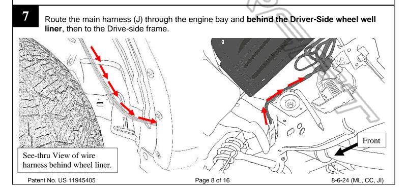
After routing all branches of the Main Harness (J), check to make sure the wires are secure with cable ties. **Be sure to avoid contact with any moving or hot engine components.** When routing wires through the wheel well area, **it is important to avoid the vehicle suspension.**
