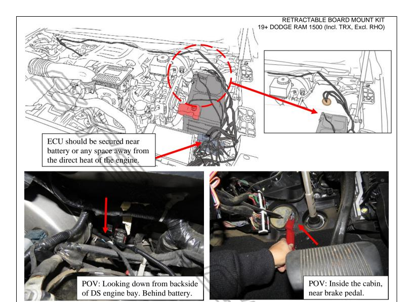
Inside the cabin, the rubber boot access is located under the steering wheel, behind the brake pedal. A pry-tool is recommended when peeling back the boot flap from the inside of the cabin.
