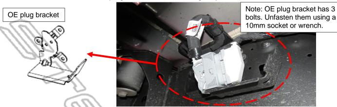
Once removed, resecure the plug to the frame out of the way of the components using zip ties.
