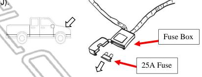
Connect the positive power lead on the main harness (J) to the positive battery terminal. Connect the negative lead to the negative battery terminal.
