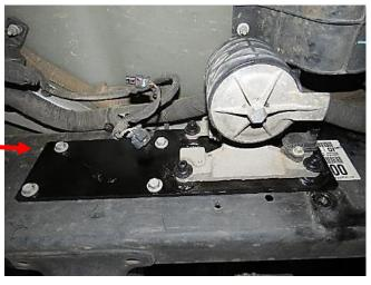
Some vehicles will have a Mass Damper instead of an ATMM. Follow the same steps and relocate the damper using the relocation brackets. Note that some vehicles will only have a mass damper on one side of the vehicle. Whenever that is the case, simply use the one appropriate relocation bracket.
