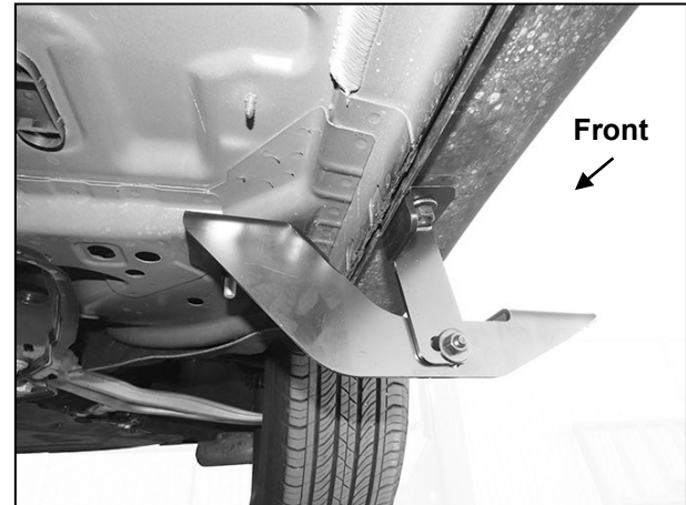
(Fig 16) Passenger/right front Mounting Brackets installed
