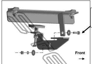
(Fig 20) Attach passenger/right center Mounting Bracket to back of Support Bracket
