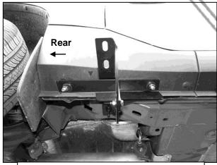
(Fig 26) Passenger/right rear Mounting Bracket and Support Bracket installed
