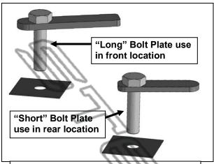
(Fig 16) Long and Short Bolt Plates with Plastic Retainers (retainer use optional)
