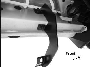
(Fig 6) Driver side front Bracket installed
