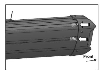
(Fig 8) Insert 8mm T-Bolts through the channel openings in the bottom of the Sidebar
