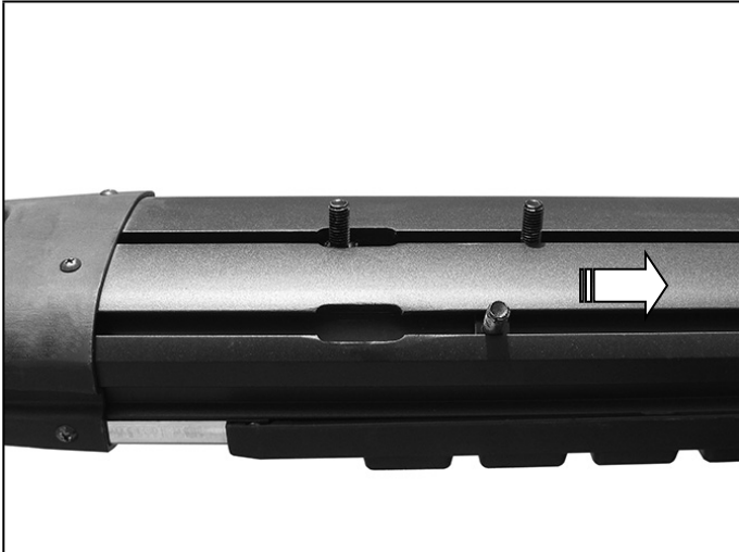
Slide (2) 8mm T-Bolts into each channel in bottom of Sidebar
