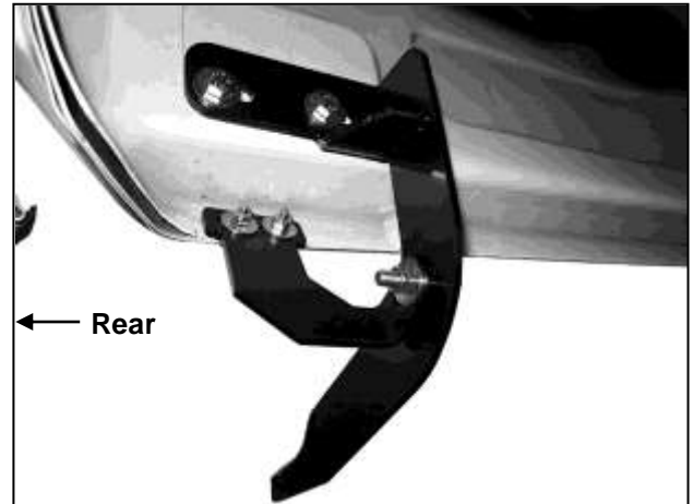
(Fig 18) Driver/Left rear Mounting Bracket assembly
