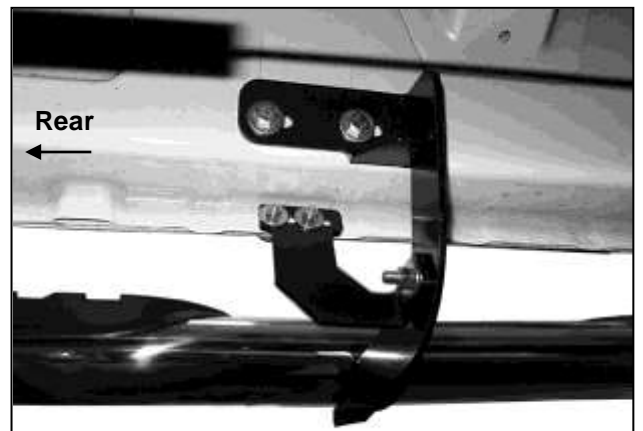
(Fig 20) Driver/left center Bracket assembly
