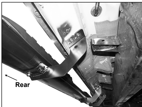
(Fig 11) Driver/left Side Bar attached to rear Mounting Bracket
