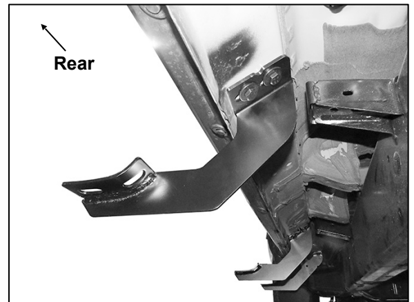
(Fig 6) Driver/left rear Mounting Bracket installed
