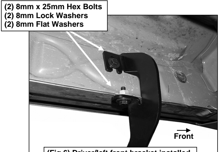
(Fig 6) Driver/left front bracket installed
