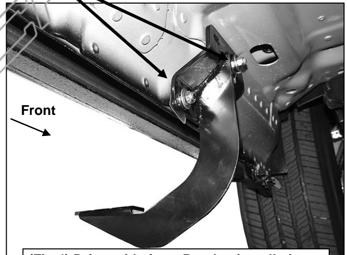
(Fig 4) Driver side front Bracket installation
