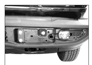
(Fig 2) Models with plastic bumper cover (see Fig 1), remove bumper pads from bumper (driver/left side pictured). Note, unplug parking sensors if equipped
