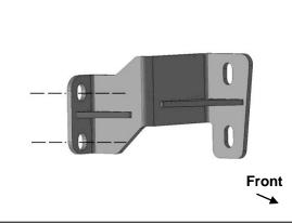
(Fig 3) Models with plastic bumper cover (see Fig 1), reuse the (2) OEM hex bolts to attach the driver/left Mounting Bracket to the front of the bumper (arrow)
