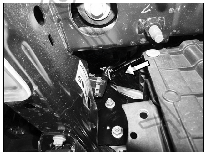
(Fig 12) Unplug all wiring harnesses leading to the front bumper (arrow). 2021-On model pictured
