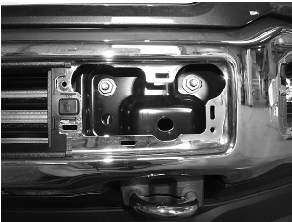
(Fig 3) 2018-20 models: From behind bumper, locate and remove bolts attaching bottom of bumper to bumper brackets. From front of bumper, remove bumper pad to locate and remove hex nuts and remove
