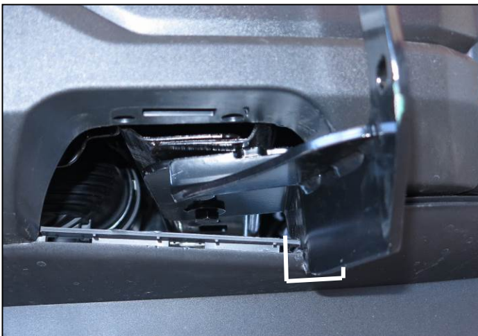
(Fig 24) 2024 models: Insert Frame Brackets and mark gusset location on bottom of bumper. Cut as required to clear brackets
