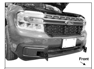
(Fig 19) Temporarily remove the Grille Guard from the Brackets.
