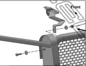
(Fig 20) Attach passenger/right Support Bracket to Grille Guard
