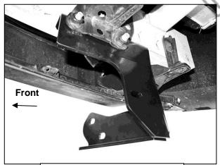
(Fig 3) Passenger/right Frame Mounting Bracket installed
