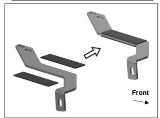
(Fig 13) Apply the Adhesive Backed Foam Pads to the passenger/right Support Bracket
