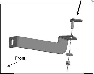
(Fig 7) Attach the Passenger/Right Support Bracket to the Bolt Plate
