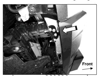
(Fig 1) Temporarily remove the (4) bolts and bent bracket attaching the bottom of the inner impact bumper to the end of the frame (arrow)
