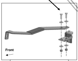
(Fig 16) Attach the passenger/right Upper Support Bracket to the top of the Mounting Bracket
