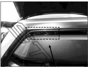
(Fig 14) Insert the flat end of the passenger/right Upper Support Bracket through the top outer opening in the grille
