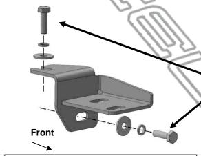
(Fig 11) Attach the passenger/right Upper Mounting Bracket to the core support
