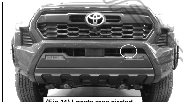
(Fig 11) Locate area circled to attach Support Bracket
