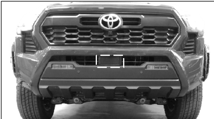
(Fig 27) Ensure the Grille Guard bar does not block or interfere with the Adaptive Cruise Control Sensor (white box)
