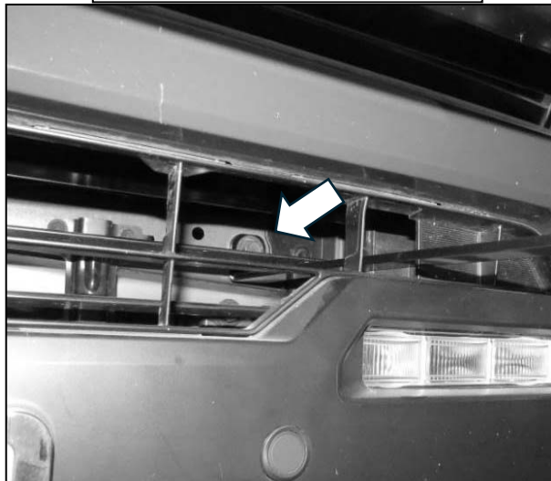
(Fig 16) Attached Support Bracket with OE bolt
