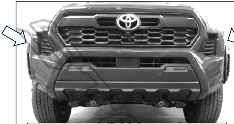
(Fig 8) With the top, bottom, and sides unclipped and unbolted, gently pull straight out on the sides (arrows) to take off the front clip.
