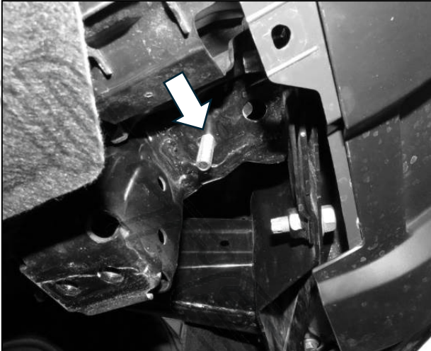
(Fig 18) Move under the driver side frame rail. Insert bolt plate into 2 nd hole from factory bumper mount. Use Plastic Retainer to keep Bolt Plate in place.
