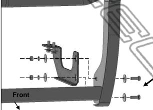
(Fig 17) Attach Grille Guard to outside of driver/left Frame Mounting Bracket
