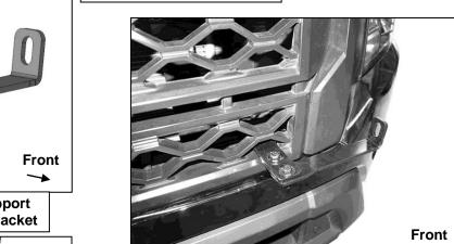
(2) 8mm x 30mm Hex Bolts(4) 8mm Flat Washers(2) 8mm Nylon Lock Nuts
