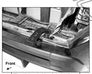
(Fig 13) Attach driver/left side Top Mounting Bracket to top of bumper
