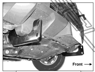
(Fig 8) Frame Brackets installed
