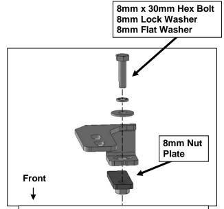
(Fig 12) Hold 8mm Nut Plate up from below steel bumper support bracket. Attach driver/left side Inner Top Mounting Bracket to top of bumper and Nut Plate
