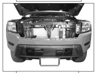
(Fig 10) Factory grille removed
