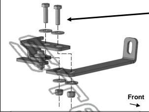
(Fig 15) Attach driver/left Top Support Bracket to bottom of Mounting Bracket
