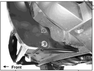
(Fig 22) Reinstall splash guard
