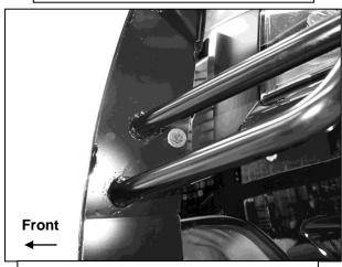
(Fig 19) Attach driver/left Top Support Bracket to inside of Grille Guard upright
